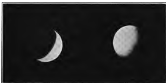
Fig. 7 — A hemispherical recess (left) and a hemispherical solid (right) lighted by a point source on the left.
